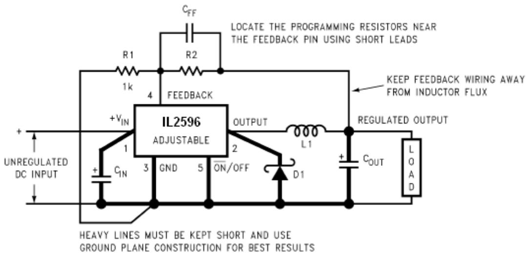
$$V_{OUT} = V_{REF} \left( 1 + \frac{R_2}{R_1} \right)$$
