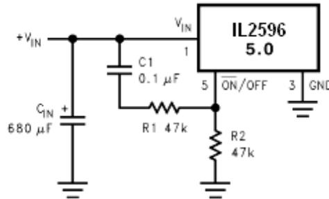
Figure 3. Delayed Startup
