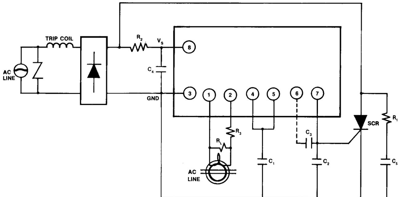
Supply voltage circuit is connected as a previous diagram. Please decide constants  $R_1$ ,  $R_2$ ,  $C_4$ , and  $C_5$  of a filter in order to keep at least 12V in  $V_s$ , when normal supply current flows.
